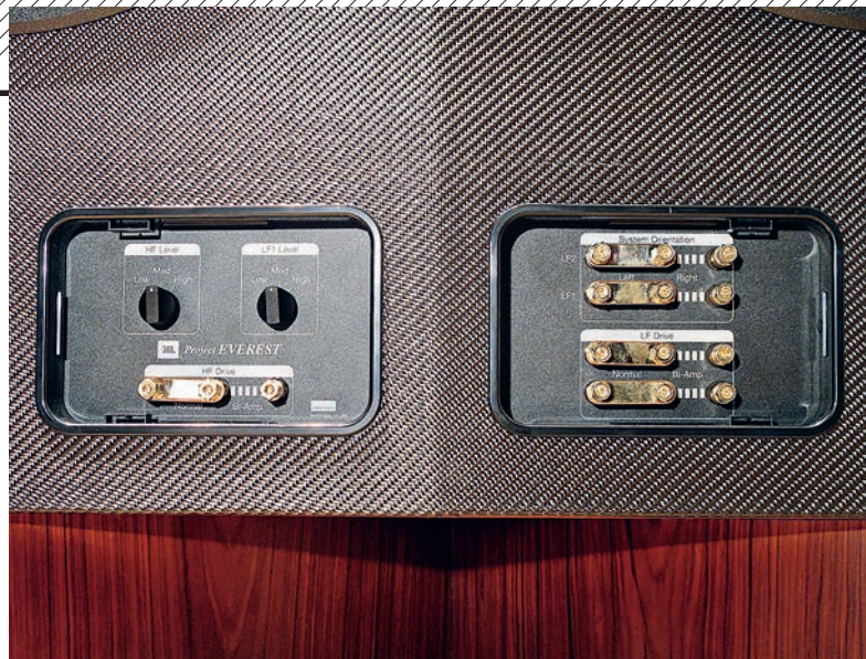
ABOVE: Cover plate on the baffle conceals switches for tweaking HF/LF levels, and links to hand the speaker and disable the network for active drive
