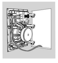
Make sure all of the speaker clamps are retracted in their "ready-tomount" position at the tops of the mount towers, tucked within the mounting opening's border.
