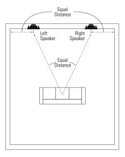
Ideally, the distance between the left and right loudspeakers should be slightly less than their distance from the primary listening area.
