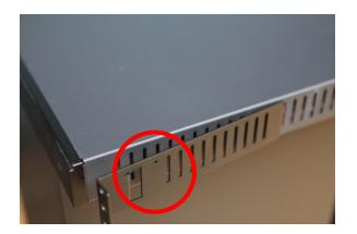
2. Insert the bracket into the amplifier's side slots. The bracket must be inserted into the back slot first (A), then the front slot (B).
