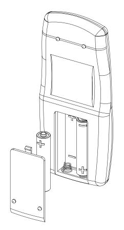
**Future Automation IR Remote** Controller needs x2 AAA batteries which are provided within the packaging.
