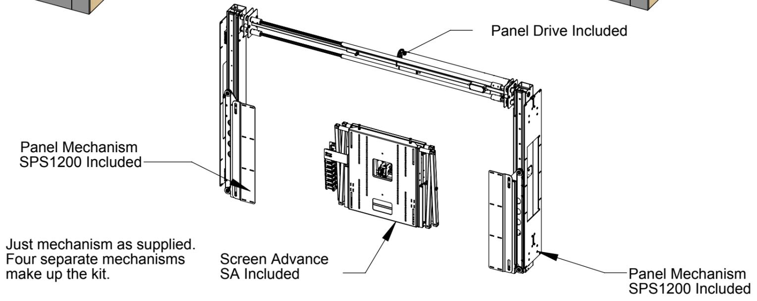
Just mechanism as supplied. Four separate mechanisms make up the kit.
