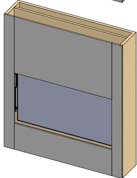
Panel lifts up/drops down to reveal TV in recess
