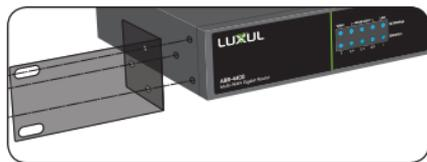
*Install Brackets for Rack-Mounting*
